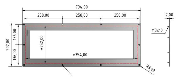
Accessory parts - VSG safety glass panel + acrylic glass panel for 2 mm front panel
